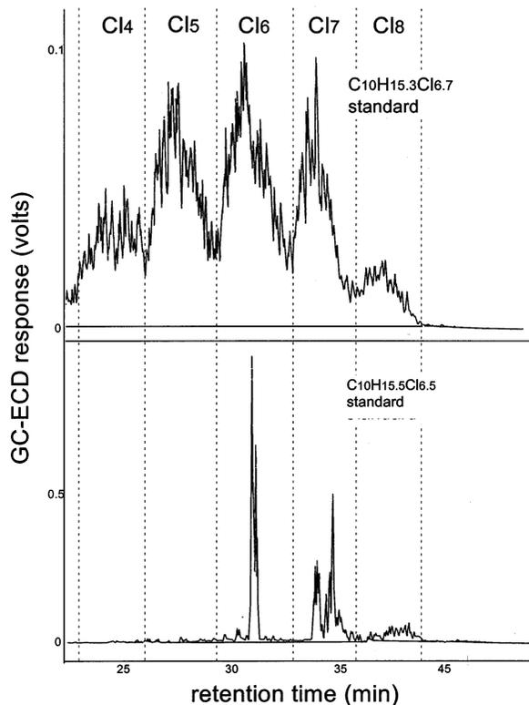
Fig. 1. GC-ECD chromatograms of the  $C_{10}H_{15.3}Cl_{6.7}$  standard (top), a free-radically chlorinated decane product, and of the  $C_{10}H_{15.5}Cl_{6.5}$  standard (bottom), a chlorinated alkene product.
