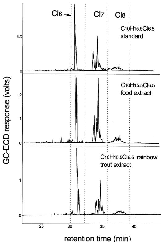
Fig. 2. GC-ECD chromatograms of the  $C_{10}H_{15.5}Cl_{6.5}$  standard (top), extracts of food spiked with  $C_{10}H_{15.5}Cl_{6.5}$  (middle), and extracts of rainbow trout exposed to the  $C_{10}H_{15.5}Cl_{6.5}$  spiked food for 85 days (bottom).
