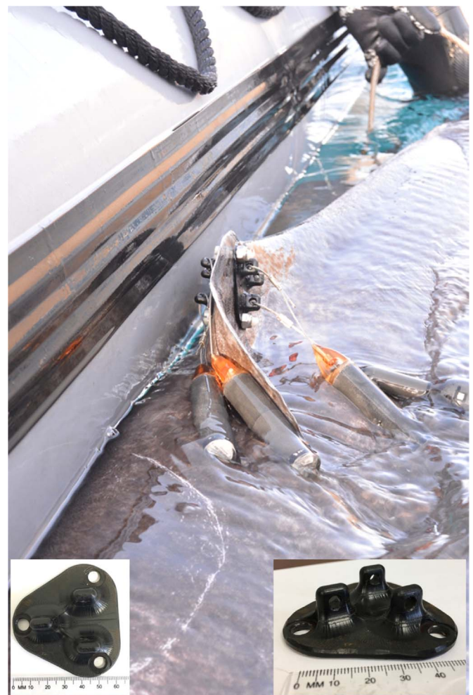
Fig. 1. Multiple mrPATs and a miniPAT attached to the dorsal fin of a Greenland shark using the designed attachment plate. Inset photographs show top down and lateral view of one attachment plate with scale bar.
