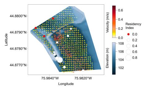
Fig. 5 Typical water velocity flow field when Edmonds Lock is not in operation, with the average water level (elevation) upstream and downstream of Edmonds Lock and Dam at 106.48 m and 103.61 m, respectively, during the study period. Arrows indicate the direction and velocity (m/s) of water flow, with arrows size- and color-graduated such that the larger and
